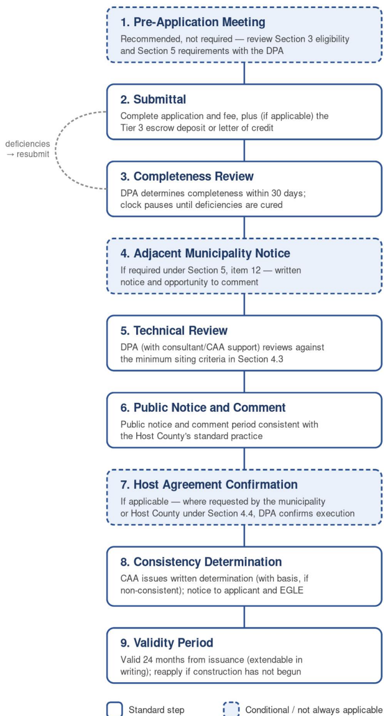
Figure 5: Siting Process Diagram
